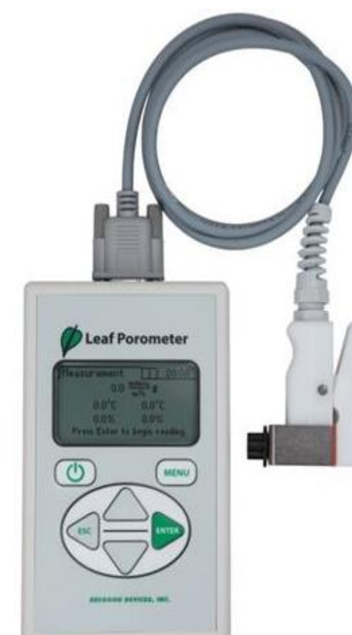
Figure 3: Porometer measuring stomata conductance (mmol/m 2 /s). The rate at which a leaf surface exchanges water vapor (H 2 O) and carbon dioxide (CO 2 ), per unit area and time.
