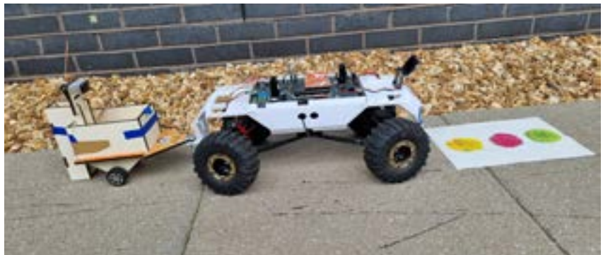
ATLAS Robot towing spot weeder, and red coloured weed
