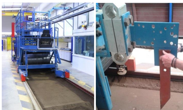
Figure 1. Soil bin processor at Cranfield University (left) and the use of a “test tine” prior to the start of the experiment (right)
